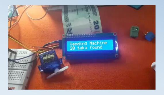
When customer presses the push button for the desired product, connected servo rotates to dispense the product
