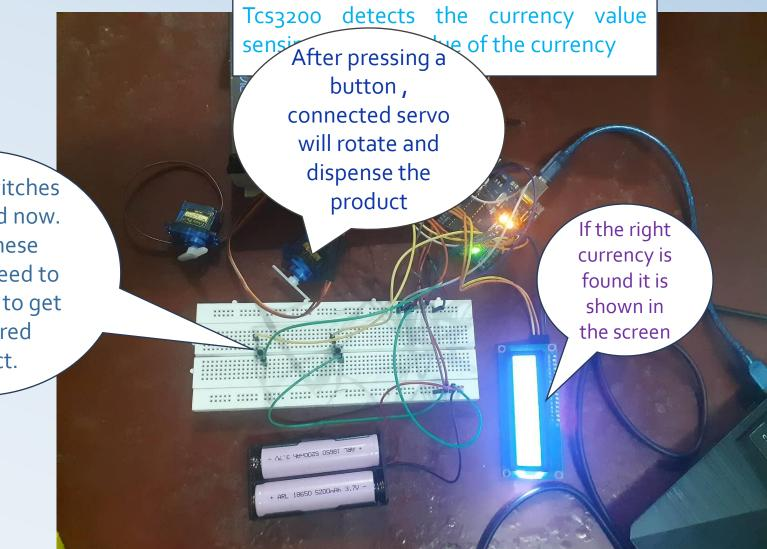
Related switches are enabled now. Any of these switches need to be pressed to get the desired product. When a customer enters a 20 taka note
