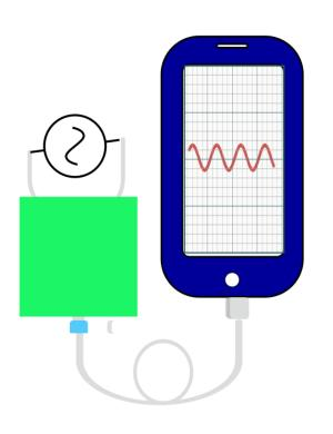
In the context of an oscilloscope, a signal generator generates some kind of signal by varying its voltage level with some frequencies, and the signal is found at the probe. Usually, the probes are in pairs, one is (let us say probe 1) phase, and the other is ground or neutral (probe 2). When two probes of the oscilloscope are connected to the corresponding probes of the signal generator, it provides the user with a real-time
